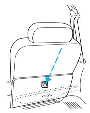
2. Lift the handle and push the seatback toward the front of the vehicle.
